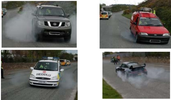
Fig 1: The diverse range of vehicles contributing to the database of deceleration ('skid') tests
