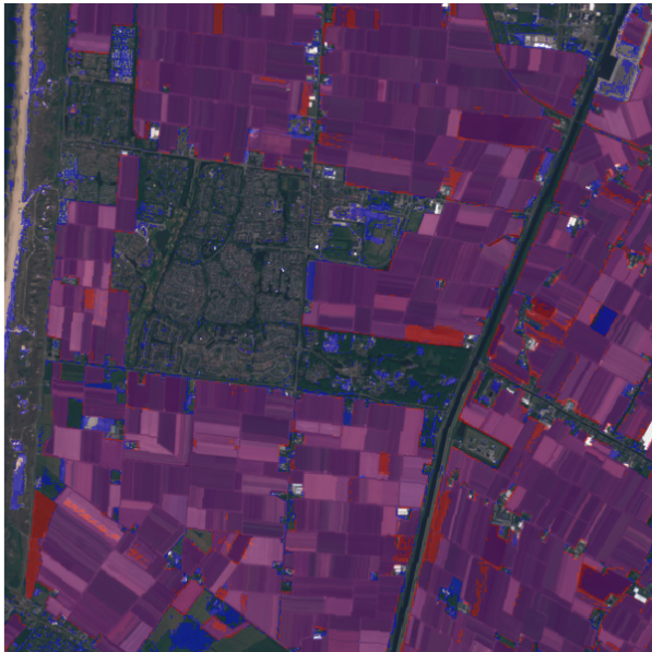
Figure 3: Graphical representation of errors in ML perceptron classification of arable land in 2017 (TP in purple, FP in blue, FN in red)
